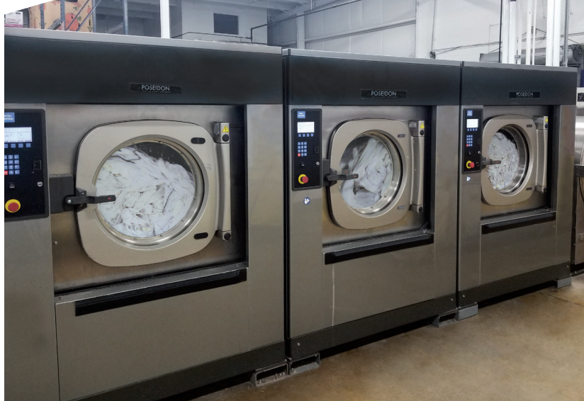
Left: The Poseidon Flatwork Ironer features an integrated folder that's significantly improved production and quality, according to Grashoff. It irons damp bed and table linens straight from the wet cleaning machines and automatically performs pre-folding. Right: The plant's Poseidon Wet Cleaning Machines are programmed with 45 unique wash programs. Each one delivers complete control over rotation action, fill levels, number of baths and rinses, water temperature, G-force extract speeds, and automatically injected chemical formulations.
