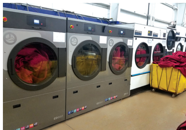
Peerless relies on a mix of Poseidon Wet Cleaning Machines and new-technology Poseidon Dryers to process textile restoration and commercial laundry work. The Poseidon Dryers cut dry time by 50 percent, according to owner Steve Grashoff.
