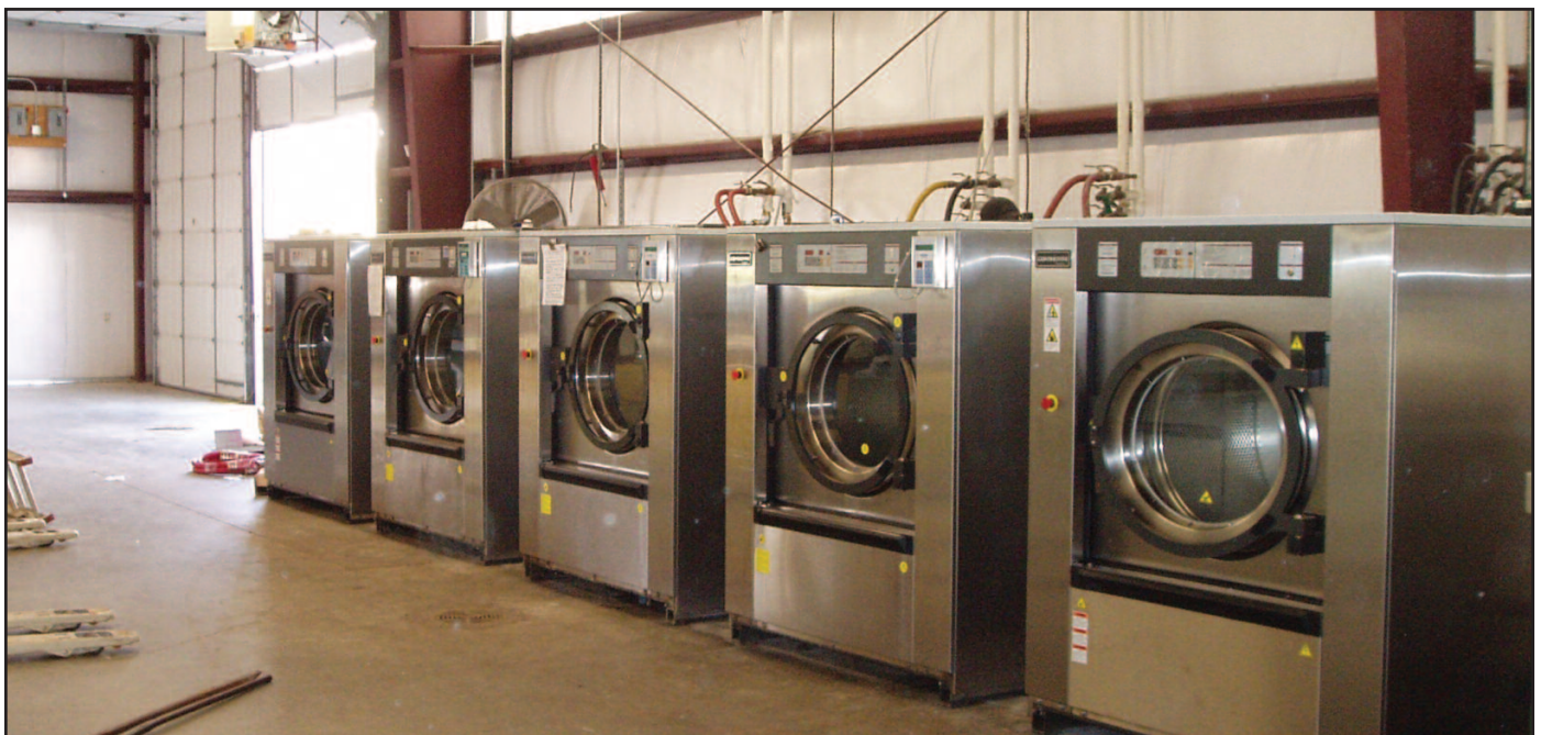
The Pro-Series Continental washer-extractors feature a soft-mount design and reach extract speeds of up to 387 G-force.
