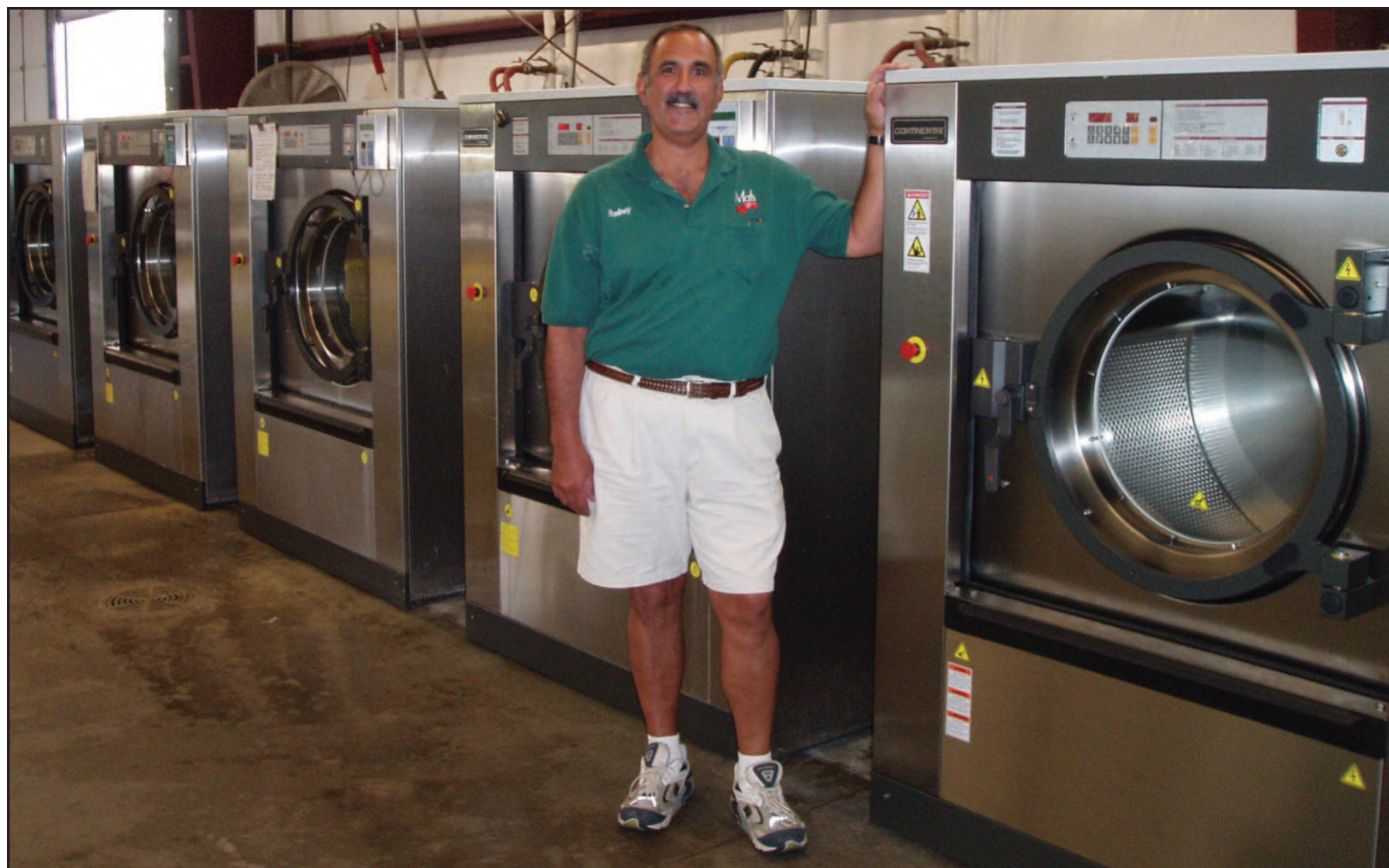
Mats for You President Rodney Rixey stands next to his new line of five 90-pound capacity Continental soft-mount washer-extractors. The soft-mount washers cut dry time from 28 minutes to 16 minutes per load—a 43.9 percent savings.
