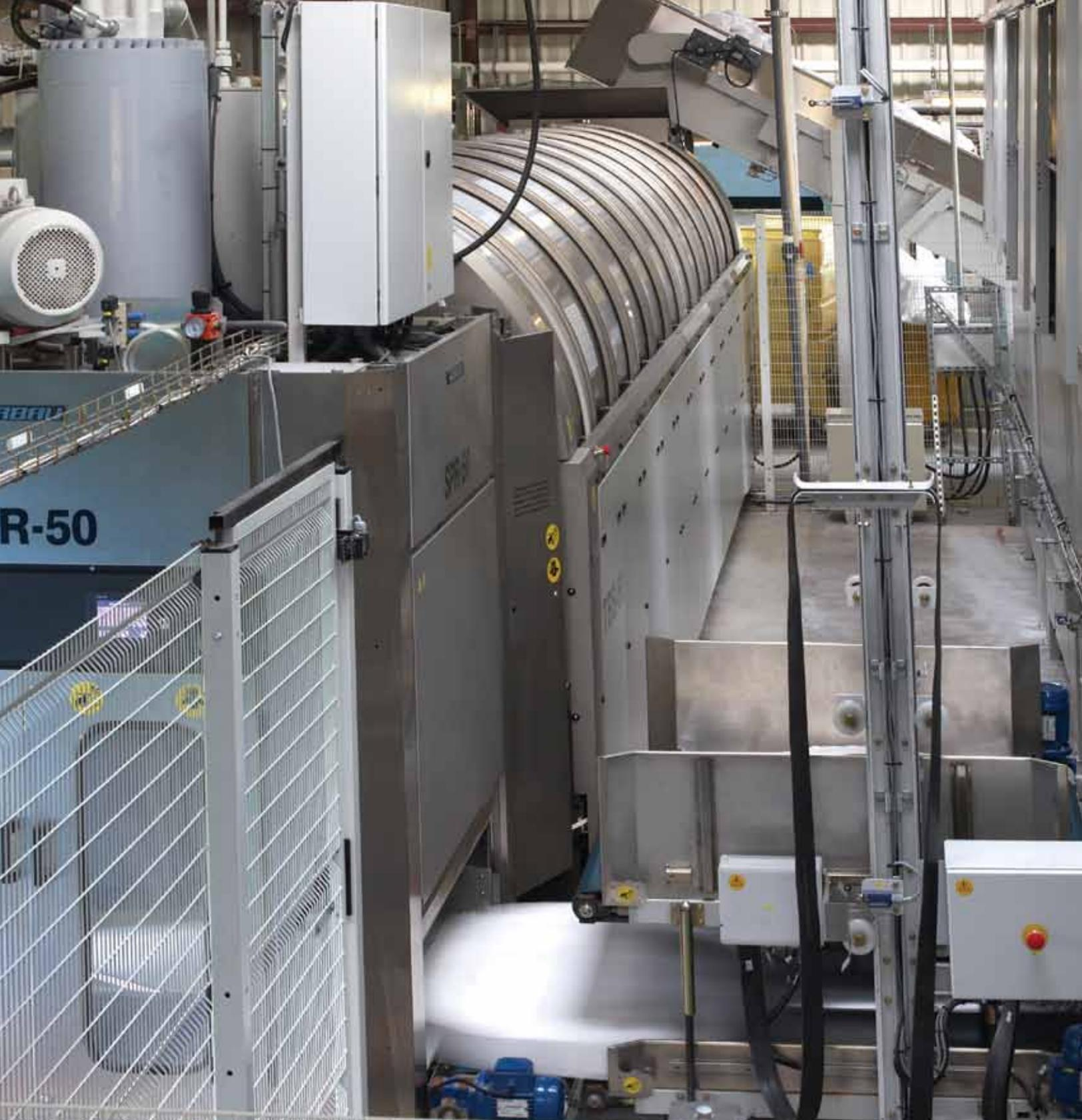
“I like everything about it. It operates off of steam, has a drain water heat reclaim system, filters, and then reuses 60 to 70 percent of the water. As the central component of the Continuous Batch Washing System, the tunnel reuses rinse and extracted water for pre-wash. Because water is recycled, less water is used and heated, lowering associated costs.”
