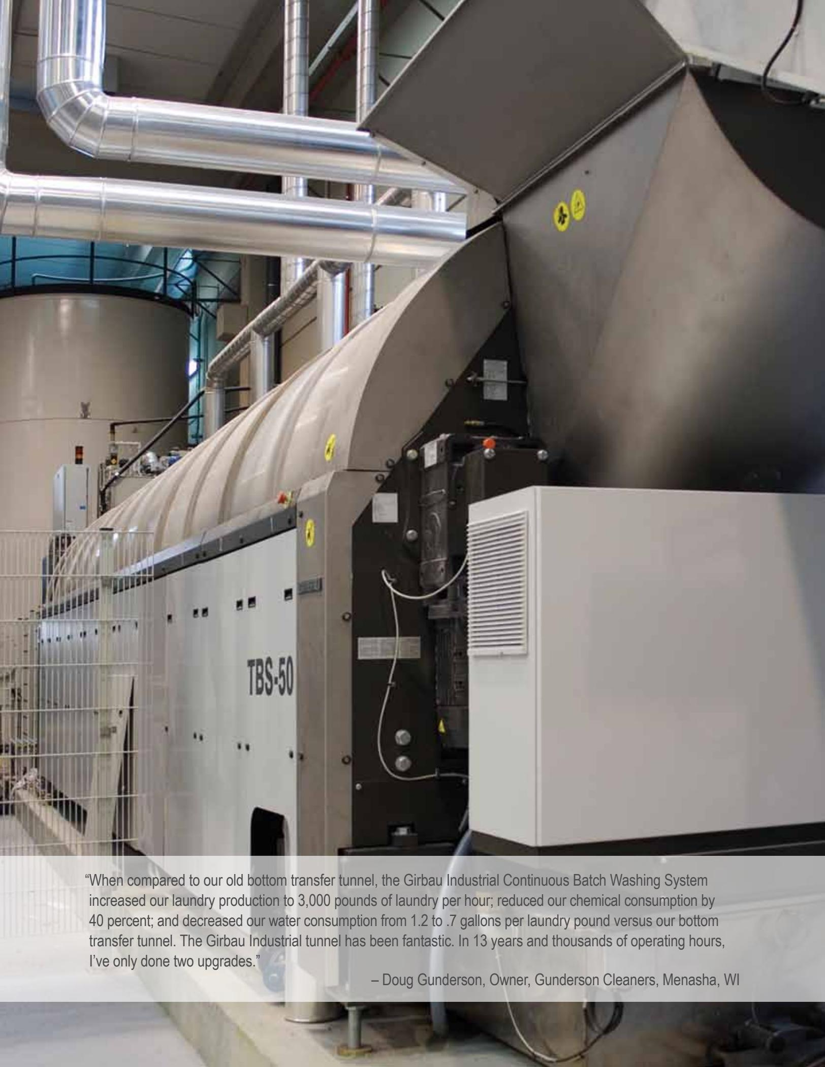
“When compared to our old bottom transfer tunnel, the Girbau Industrial Continuous Batch Washing System increased our laundry production to 3,000 pounds of laundry per hour; reduced our chemical consumption by 40 percent; and decreased our water consumption from 1.2 to .7 gallons per laundry pound versus our bottom transfer tunnel. The Girbau Industrial tunnel has been fantastic. In 13 years and thousands of operating hours, I’ve only done two upgrades.”
