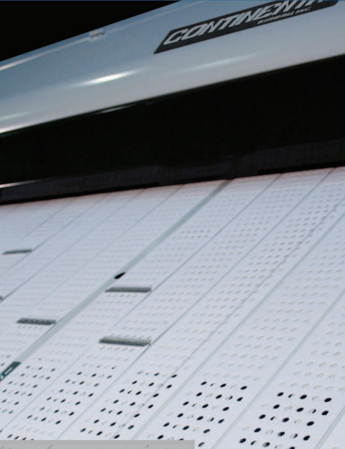
Engineered for medium- and high-volume laundries where space is at a premium, the Compact 5-in-One Ironing System not only features a compact design, it quickly feeds, irons, folds, stacks and accumulates at speeds of up to 50-feet-per-minute.
